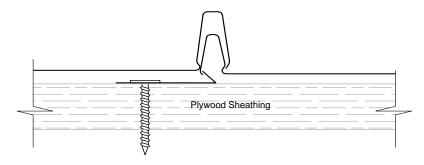
The reversing strip allows the Easy-Lock panels to be installed working both left and right. The reversing strip is most commonly used on hip roof applications although it can be used on other roof styles.
