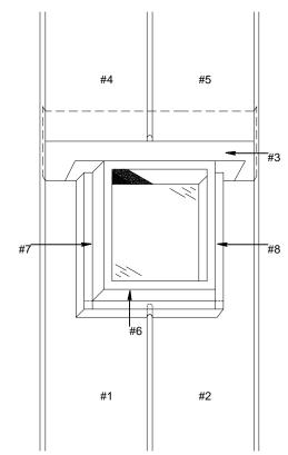
Diagram of part placement around the skylight.
