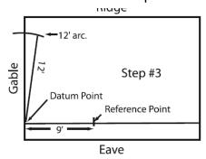
**Step 4:** From the reference point make a 15-foot arc to intersect the 12-foot arc. Snap a chalk line from the intersection point to the datum point. You now have a straight edge to align your first panel along the gable.
