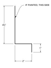
Apply parts as described on the following pages. Please note that the 12-inch leg of the pan flashing used on a chimney application will need to be bent to the pitch of the roof.
