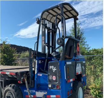
Mounted on the rear of a carrier vehicle, the truck-mounted "piggy-back" forklift will accompany you right to your place of use, opening up unprecedented possibilities in terms of transportation. It can travel sideways, carrying panels up to 40' long, allowing delivery in locations that would typically be considered impossible to reach.
