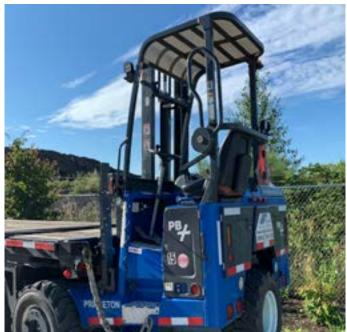
Mounted on the rear of our semitrailer, the truck-mounted "piggy-back" forklift will accompany you right to your place of use, opening up unprecedented possibilities in terms of transportation. It can travel sideways, carrying panels up to 40' long, allowing delivery in locations that would typically be considered impossible to reach.
