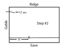
**Step 3:** Measure 9 feet from the datum point along the alignment line and establish a reference point there.
