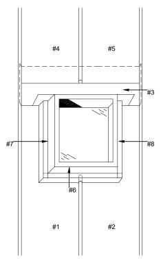
Diagram of part placement around the skylight.
