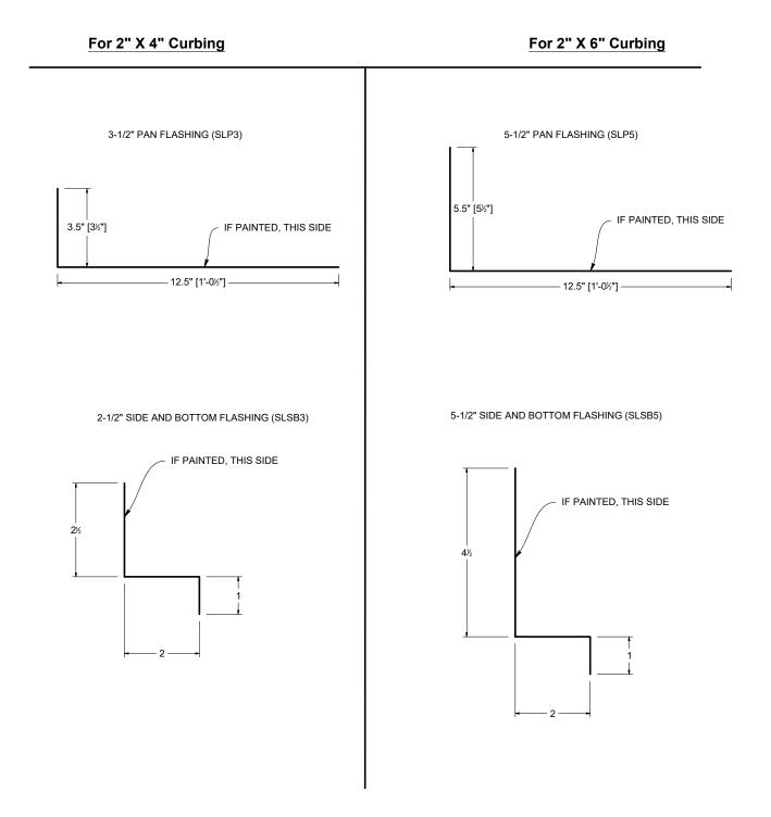
Apply parts as described on the following pages. Please note that the 12-inch leg of the pan flashing used on a chimney application will need to be bent to the pitch of the roof.
