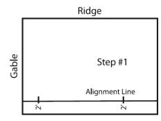
**Step 2:** Start from a point (datum) on the alignment line 1/4" to 1/2" from the left (or right depending on which edge you're starting from). Establish a 12' arc from datum point.
