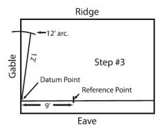
**Step 4:** From the reference point make a 15-foot arc to intersect the 12-foot arc. Snap a chalk line from the intersection point to the datum point. You now have a straight edge to align your first panel along the gable.
